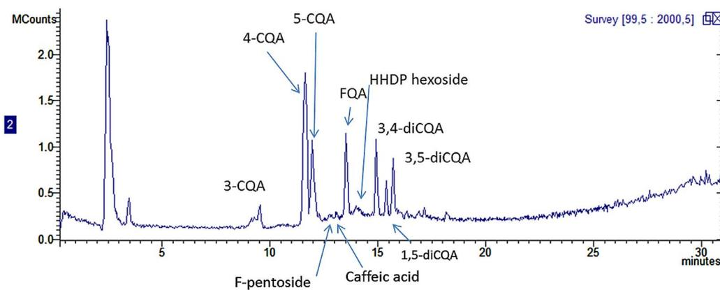
Fig. 2. Representative chromatogram obtained from HPLC-MS/MS analysis of GCBE in negative ion mode.
